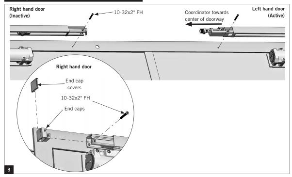
NOTE: EXAMPLE: Left hand active door shown. For right hand active installations, install active track assembly on right hand door and inactive track assembly on left hand door.
