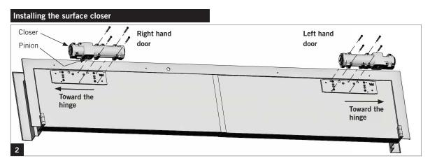
NOTE: Orient pinion closest to hinge.
